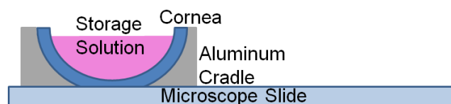
Figure 16. Cornea cradle diagram. Reprinted with permission from W. Calhoun, R. Weiblinger, A. Beylin, and I. K. Ilev, "Assessing the phase retardation in corneal tissues using a femtosecond laser," Rev Sci Instrum , vol. 84, p. 084301, Aug 2013. Copyright 2013, AIP Publishing LLC.
